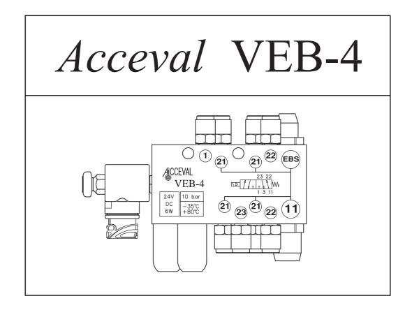
Lift Axle Control Valve Electrically Commanded From EBS System
